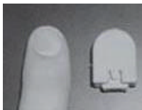
Figure 3-9. A V1220 Speaker actuator made by Audiologic Engineering. A finger is included for scale.
