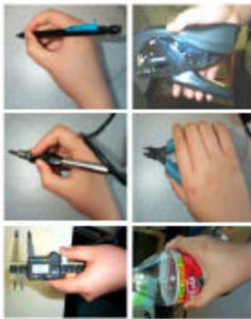
Figure 3-13. Precision grip vs. strength grip.
