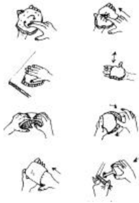
Figure 2-4. Typical movement patterns for EPs described by Klatzky and Lederman. From top left counter clock wise: lateral motion, static contact, enclosure, function test, part motion test, contour following, unsupported holding and pressure. –from p.346 (Klatzky 1993)
