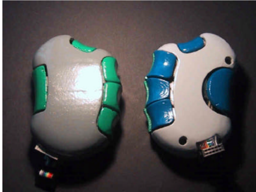
Figure 3-18. A working set of ergonomic ComTouch allowing users to use five channels of vibrotactile communication
