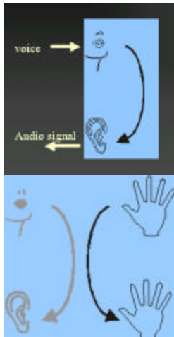
Figure 3-2. Addition of a tactile modality to existing communication. ComTouch proposes the addition of a new modality; touch, onto an existing interaction to increase the shared sensory experience in audio communication.
